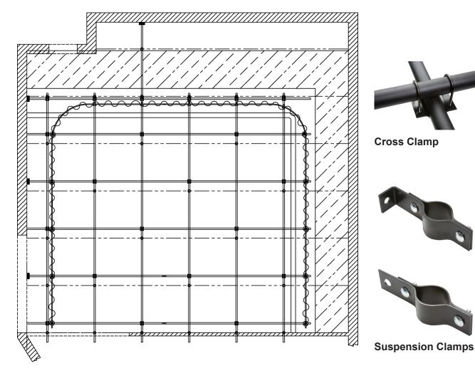
SSRC manufactures studio pipe grid systems using 1 1/2" schedule 40 pipe, 90° cross clamps, wall flanges and suspension clamps (all-thread or chain).
